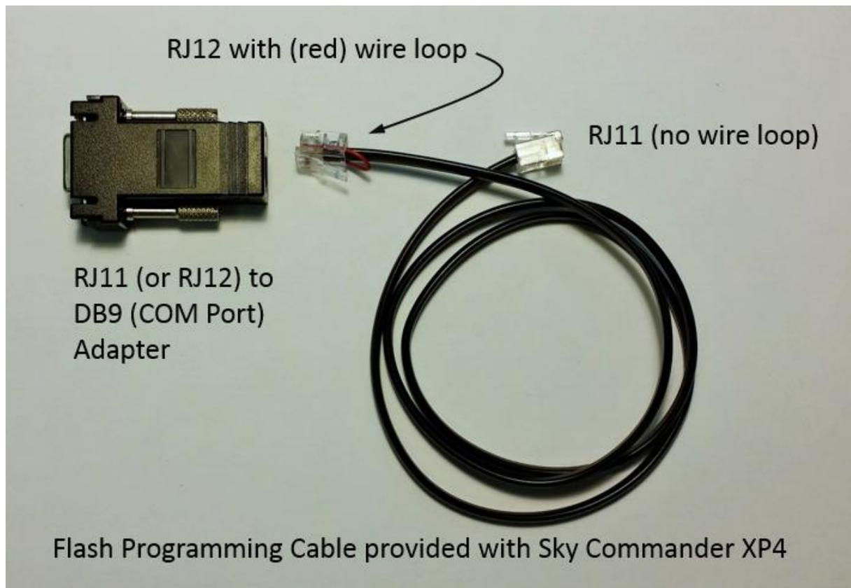
You may also need a USB to serial converter cable if your PC does not have a COM port (most new ones don't). These are readily available and inexpensive – do a web search for “USB to Serial Adapter”. Any of them should work fine.
