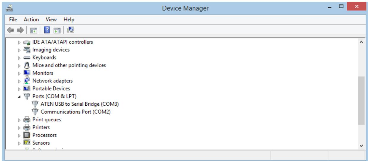
Device Manager under the Control Panel in Windows will help you determine this. In the example above, a USB to Serial Port converter cable was plugged into the PC and it appears as COM3.
